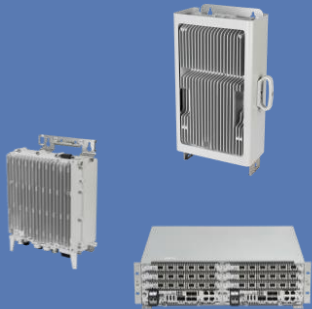
AirScale Base Station: Multi-band radio + Baseband Units
